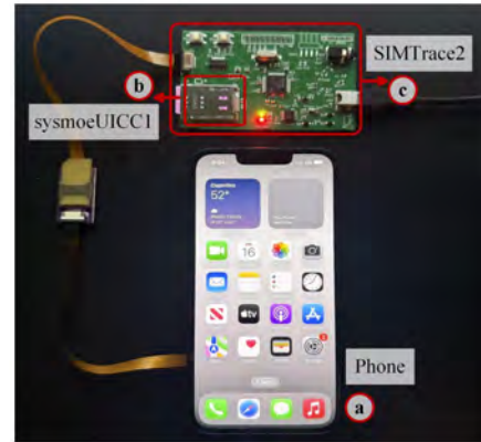
Figure 4: Setup for capturing proactive communication: (a) iPhone 13, (b) sysmoEUICC1 for downloading the eSIM, (c) SIMtrace2 for capturing communication between the phone and the eSIM profile.
